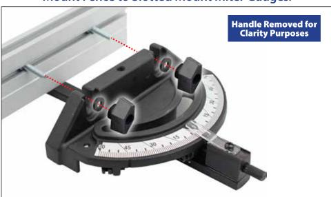
Some miter gauges come with slots instead of holes. Simply guide the bolts into the slots and secure the miter fence to the miter gauge using the supplied bolts, washers and t-knobs.
