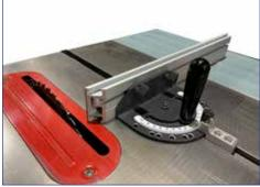
Once the fence is mounted to your miter gauge you can adjust the placement of the fence by simply loosening the knobs and sliding the fence into the desired position. Make sure that you leave at least 1/4" of space between the fence and the blade. Once adjusted, make sure you secure the fence in place by firmly tightening the knobs.
